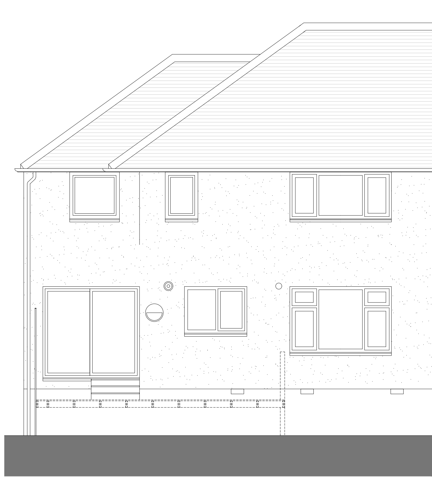
REAR ELEVATION scale 1:50
